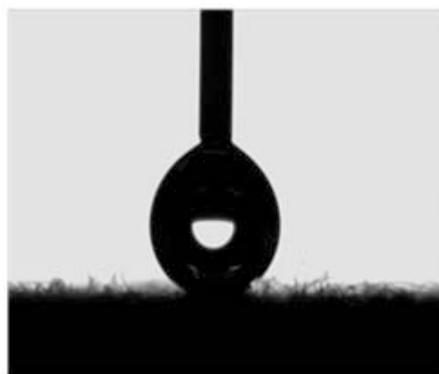
Fig. 1 Water droplet on the superhydrophobic surface of a PFPE functionalized CC
